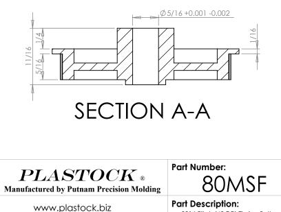
.0816 Pitch (40 DP) Timing Belt Pulleys For Belts up to 1/4" Wide
